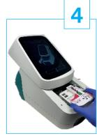
Insert cartridge into the instrument
